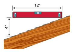
280. The slope of the roof shown here is measured with a 12" level and a ruler. What is the slope of this roof?
